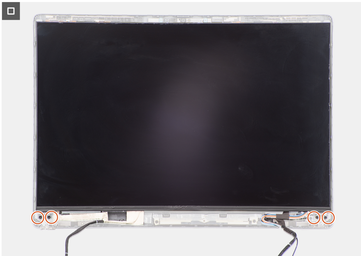
Figure 73. Installing the display panel
