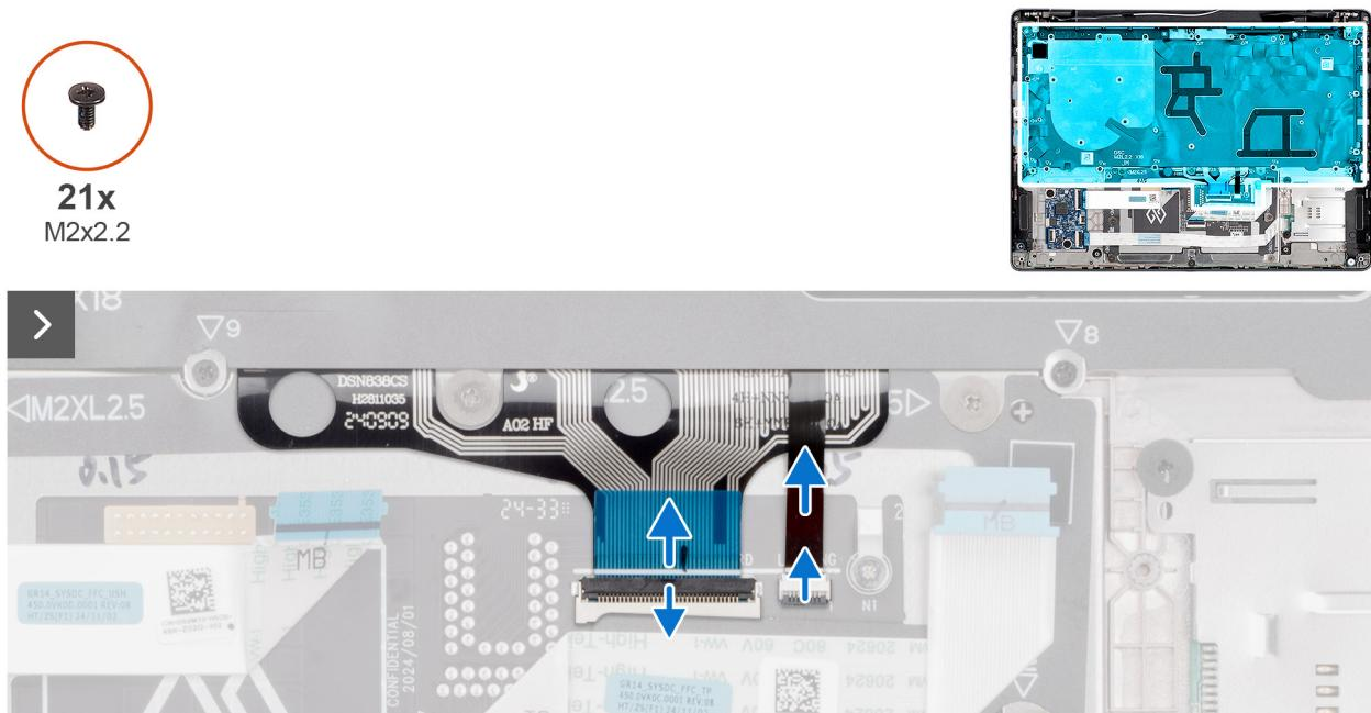
**Figure 80. Removing the keyboard**
