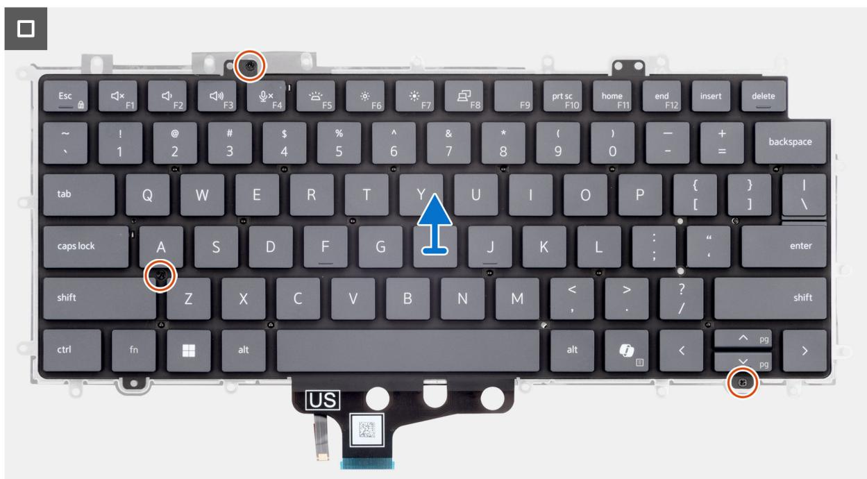
Figure 82. Removing the keyboard
