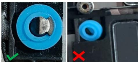
**Figure 28. Installing the speakers**
