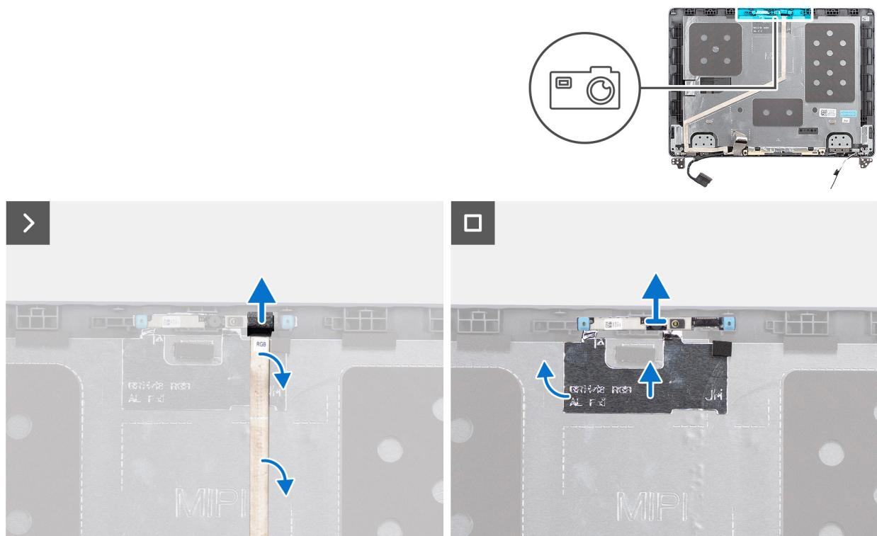
**Figure 66. Removing the camera**
