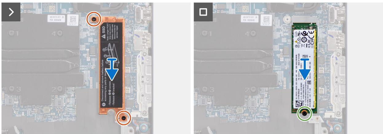
**Figure 22. Removing the M.2 2280 solid state drive**
