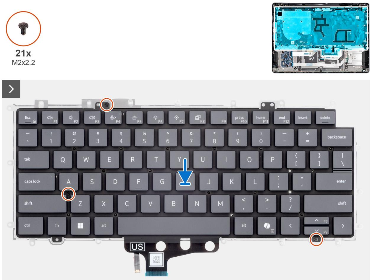
**Figure 83. Installing the keyboard**
