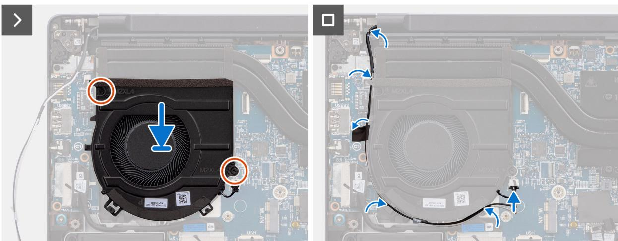
**Figure 30. Installing the fan**
