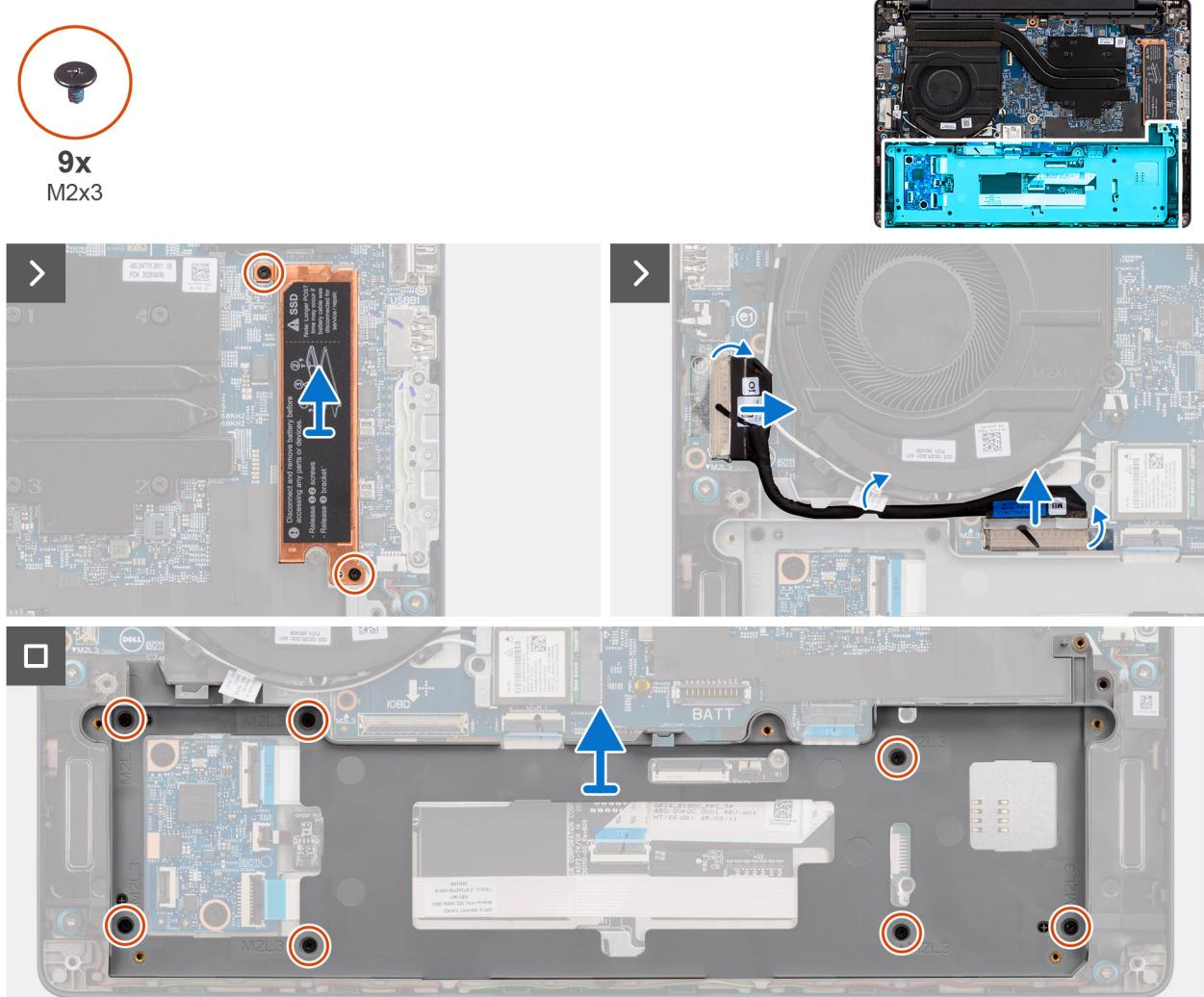
**Figure 31. Removing the battery frame**
