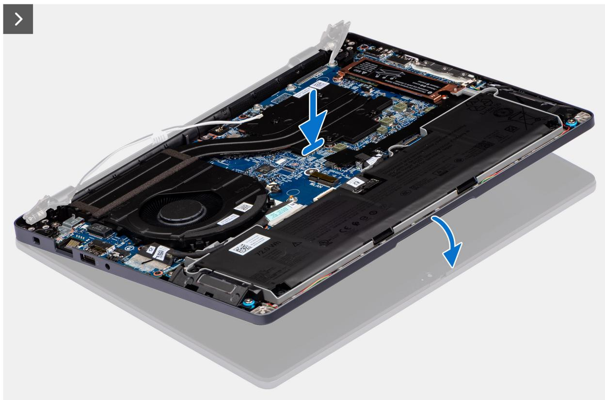
**Figure 46. Installing the display assembly**
