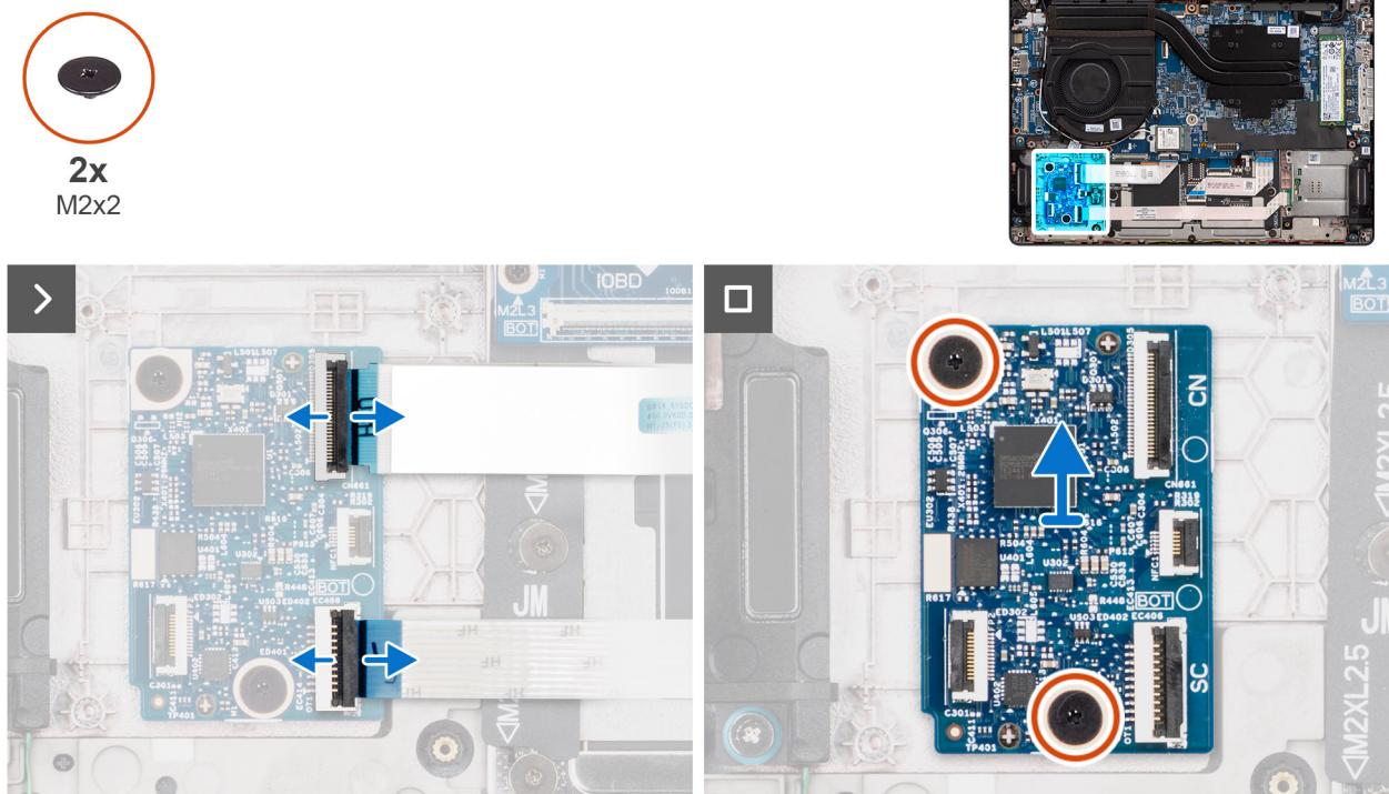
**Figure 33. Removing the USH board**
