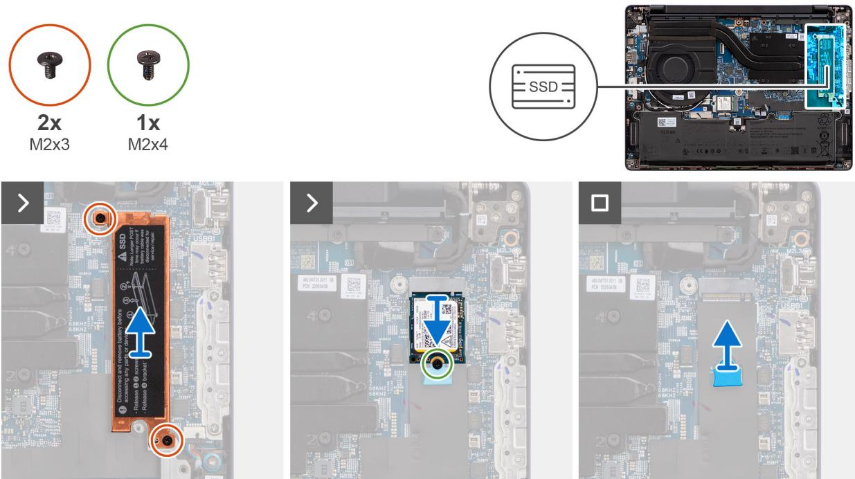
**Figure 20. Removing the M.2 2230 solid state drive**
