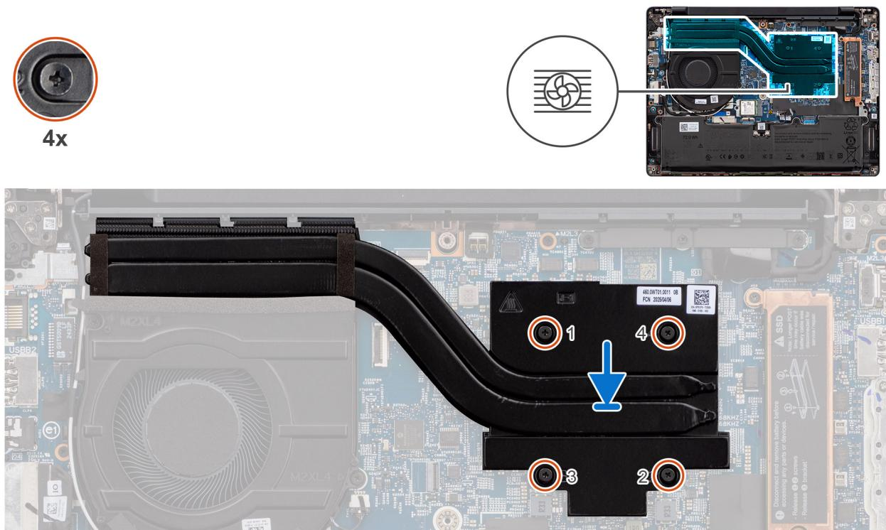
**Figure 38. Installing the heat sink**
