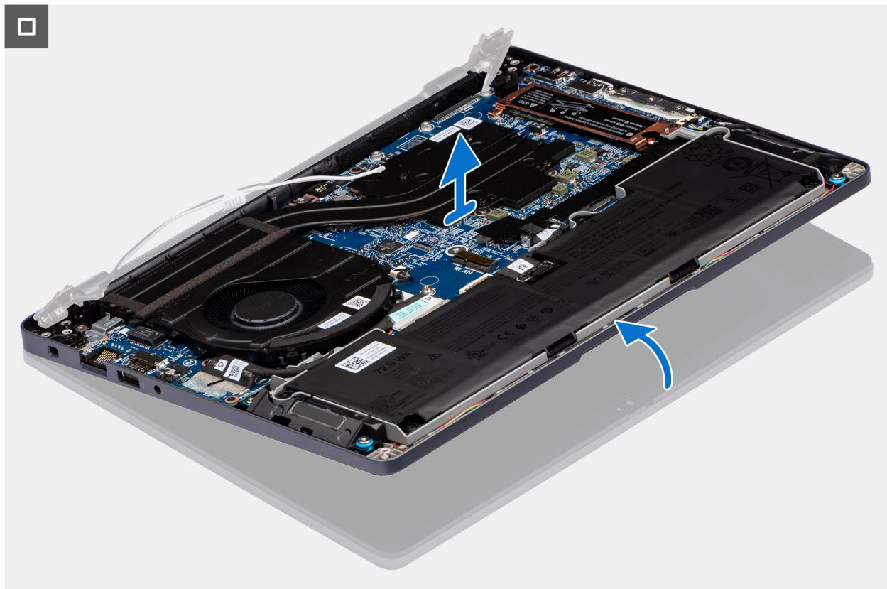
**Figure 44. Removing the display assembly**
