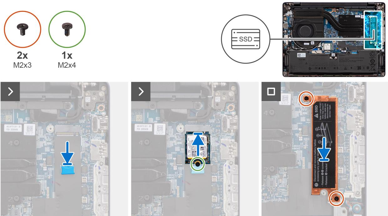
**Figure 21. Installing the M.2 2230 solid state drive**
