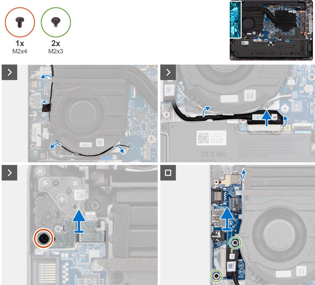
**Figure 39. Removing the I/O board**
