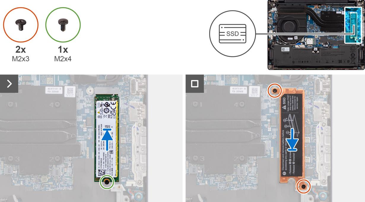
**Figure 23. Installing the M.2 2280 solid state drive**
